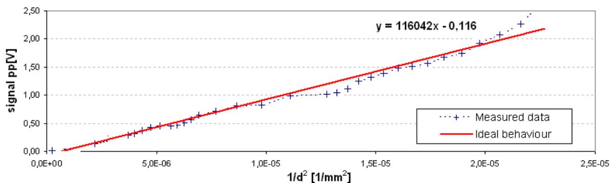
**Figure 1:** Detector's functional dependency on the distance of the IR source
