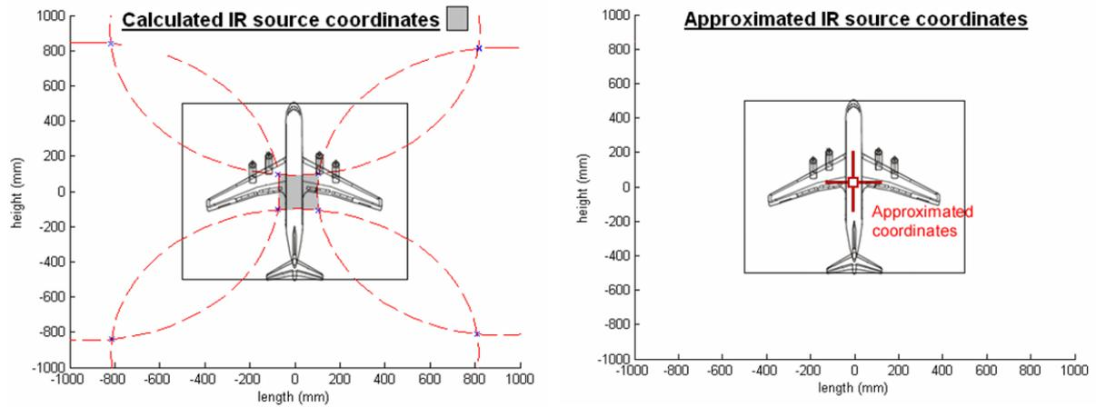
**Figure 3:** Comparison of the localization accuracy using a) MOC b) ANN
