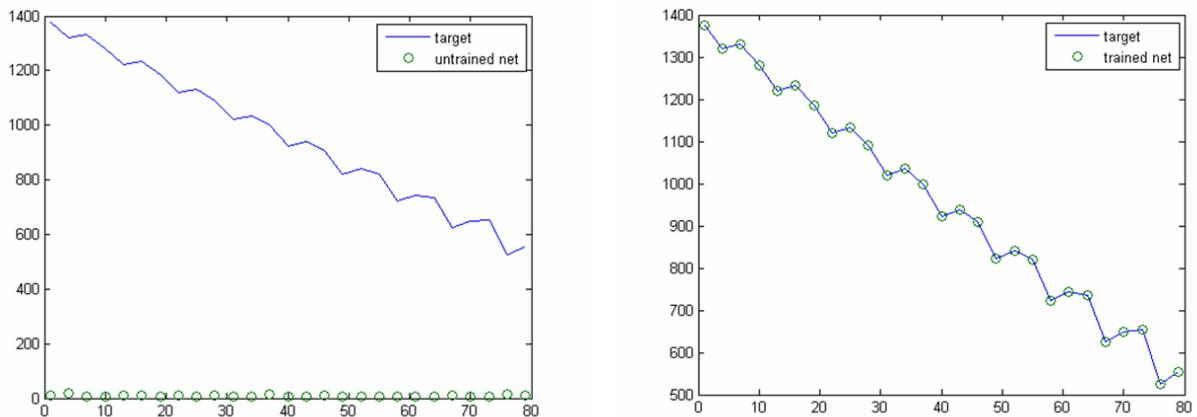
**Figure 2:** Performance graphs of the a) untrained and b) trained network
